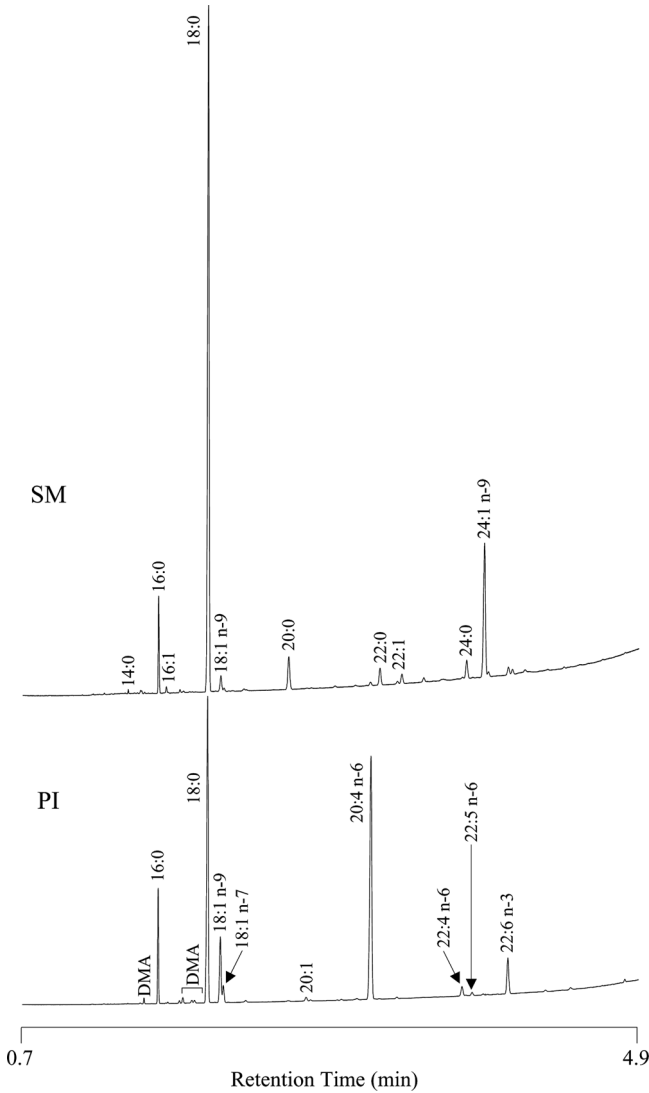
Figure 3. Fast GC trace of fatty acid methyl esters (FAME) prepared from purified brain sphingomyeline (SM) and phosphatidylinositol (PI).
